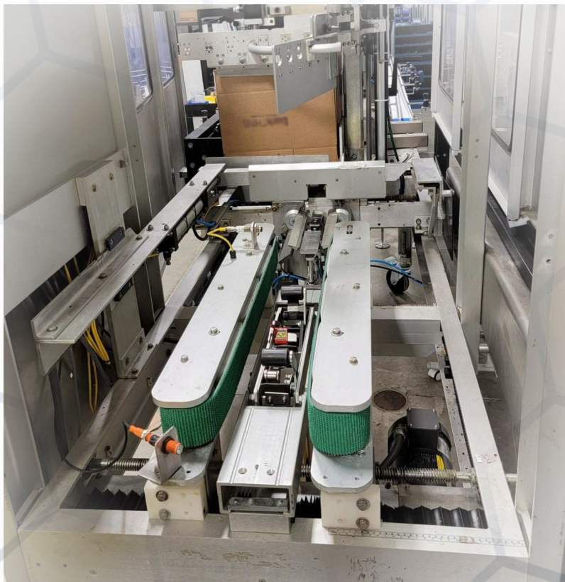
Uni-drive synchronized side belt conveyor system
