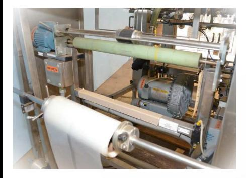
Bags are cut from a roll of gusseted polyethylene layflat tubing. A 26" long heated cutoff bar forms bags of variable lengths.
